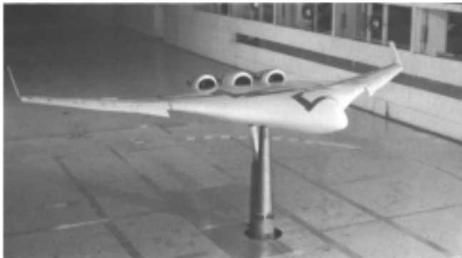
Figure 25. Wind tunnel model of a blended wing-body configuration.
