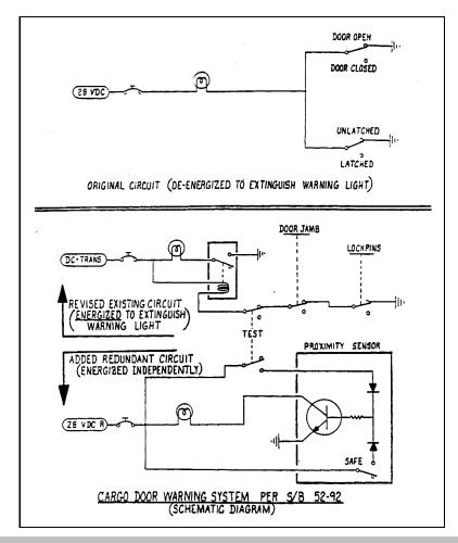
Figure 3.--Cargo door warning switch electrical diagrams.
