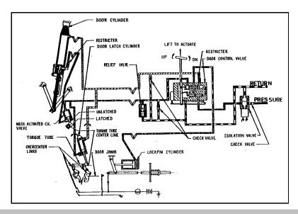
Figure 1.--Hydraulic routing within the cargo door hydraulic system.
