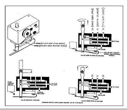
Figure 2.--Main cargo door components.
