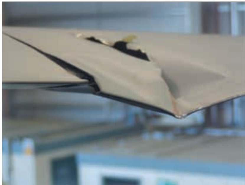
Photo No. 2 - Damage to White Blade
