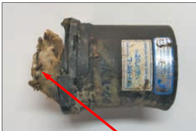
Altimeter No. 1 with broken mounting screw
