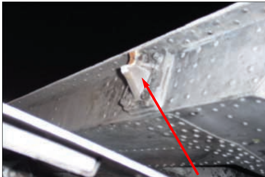
Photo No. 1: The broken half-hinge attached to the undercarriage door.
