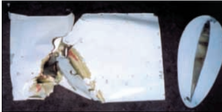
Three sections of the RH stabilizer found 0.5 miles from the landing site
