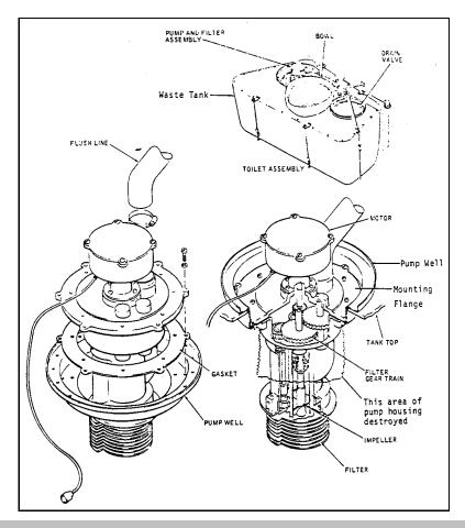
Figure 11.—Lavatory pump and filter system.
