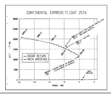
Figure 4.--Radar-derived descent profile.
