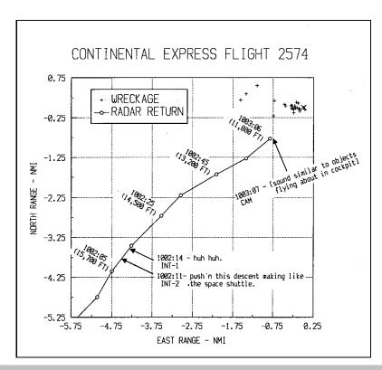
Figure 2.--Radar-derived ground track, CVR sounds, and wreckage distribution.
