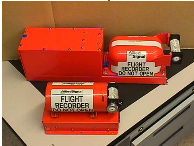
Figure 7 - Physical Size Reduction of Crash Recorders
