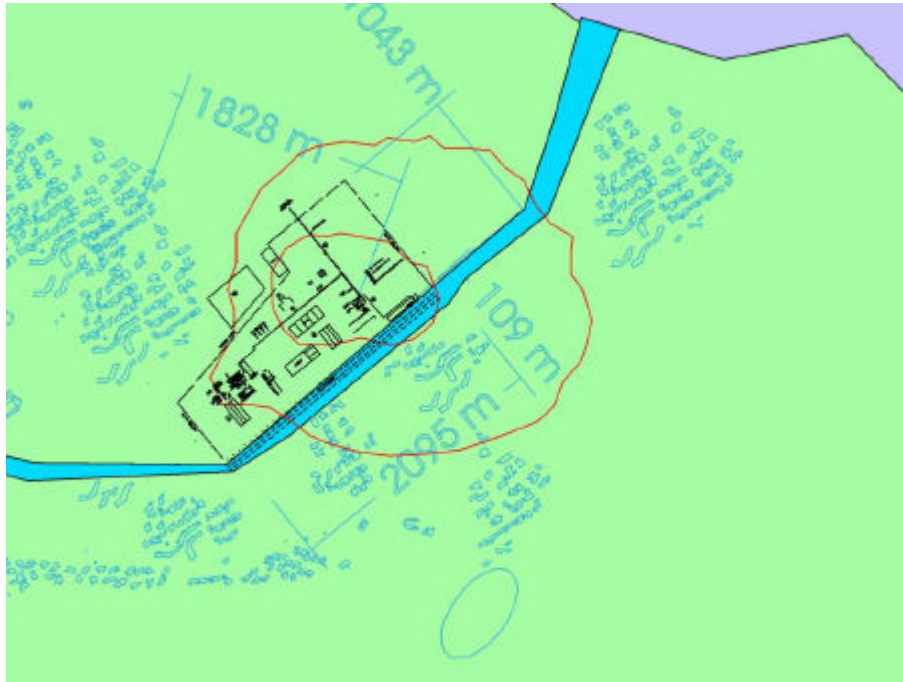
Figure 1. Discrepancy in the results of individual risk calculations relevant to risk-informed Land Use Planning: Maximum and minimum distances for the isorisk curve 10^{-5} yr ^{-1}
