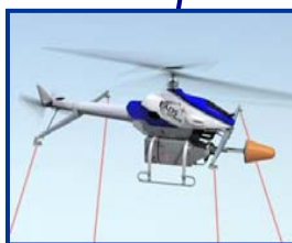
Near-field Probe on Remote Controlled Airborne platform
