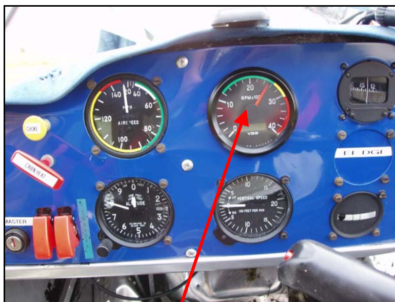
Photo 2. Tachometer frozen at approximately 2,550 RPM following impact
