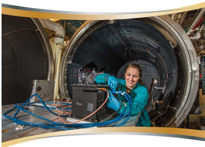
Researcher prepares a global burst detector subsystem for a test in the flight test chamber at Sandia National Laboratories in Albuquerque, N.M., August 4, 2016. (Photo by Randy Montoya)
