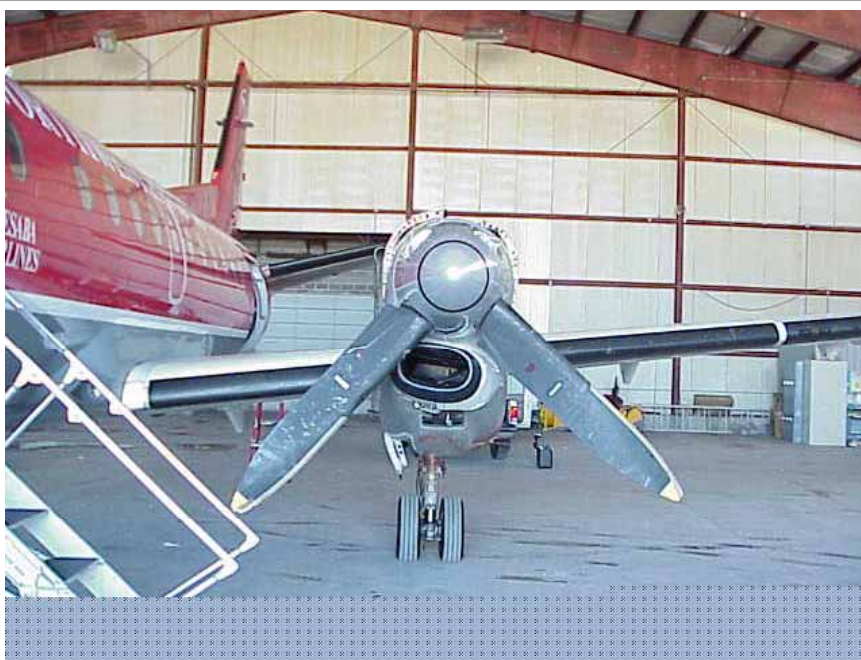
This Saab 340 hit two deer when landing at a Michigan airport, April 2000. The engine was torn from its mountings and is being held in place by the oil and fuel lines only. (Photo courtesy Northwest Airlines)
