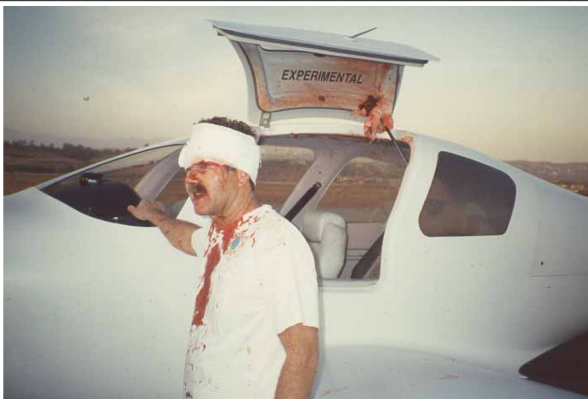
A gull penetrated the windshield of this experimental aircraft shortly after take off from a California airport, November 1998. The pilot suffered severe head lacerations. (Photo by J. R. Dodd, Airport Manager)
