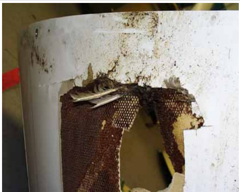
This radome on a Boeing-767 suffered extensive damage when the aircraft struck a bird, December 1999. Note the feathers caught at the top of the puncture. (Photo courtesy B. Mackenzie)
