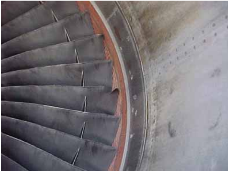
This is a close up of one engine from a Boeing-757. A flock of several hundred European starlings flew in front of the aircraft at rotation from a midwestern airport, February 1999. One engine was destroyed and the other damaged. Over 400 dead starlings were picked up from the runway area following the strike. (Photo courtesy local airport authority.)
