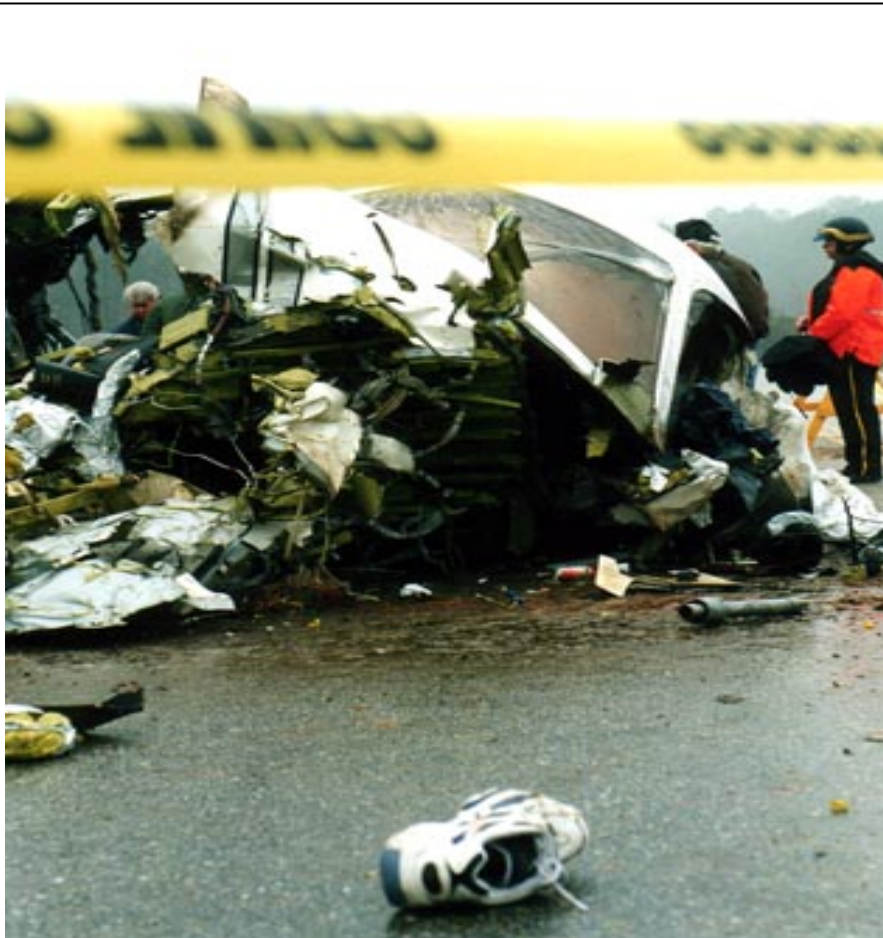
A Learjet 60 landing at Troy, Alabama Municipal Airport on 14 January 2001 collided with two white-tailed deer which disabled the thrust reversers. The aircraft ran off the end of the runway into a ditch and burst into flames. The pilot and first officer had serious injuries and were flown to a hospital. Cost to replace aircraft was $9.5 million. Other costs totaled $25,000. Photo courtesy The Messenger, Troy, Alabama.
