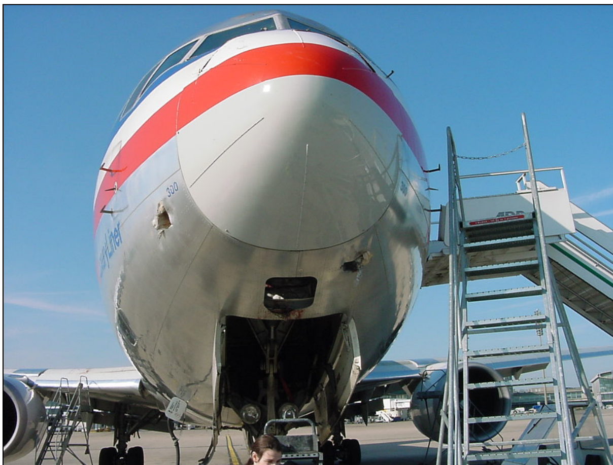
A Boeing 767 operated by a U.S. air carrier struck a flock of migrating northern shovelers while climbing through 14,000 feet on departure from an airport in France, April 2001. The strike caused 11 punctures to the aircraft. One bird penetrated the cockpit, causing depressurization and splattering crew with bird debris and insulation. The pilot had to use an oxygen mask. Aircraft returned safely to airport. Cost of repairs was over $1 million. Photo courtesy of the airline.
