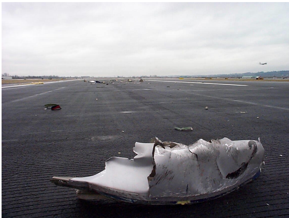
An MD-11 with 217 passengers ingested a herring gull into the #3 engine on departure from a west coast airport in January 2001. The engine stall blew off the nose cowl that was sucked back into the engine and shredded. The engine had an uncontained failure. The pilot aborted take off and blew two tires.
