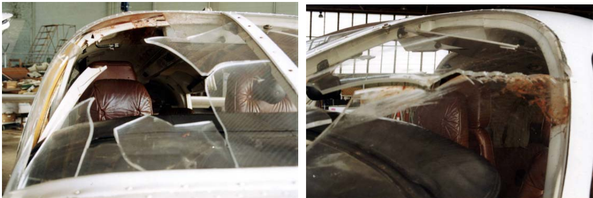
A Piper 34 aircraft struck two red-breasted mergansers at 800 feet AGL at night (21:25 local time) on approach to a southern USA airport on 9 March 2003. The birds penetrated the left and right windshield panels. The pilot was able to land the plane safely. Feather remains were identified by the Smithsonian Feather Identification Lab. (photos provided by Air Reldan, Inc.)
