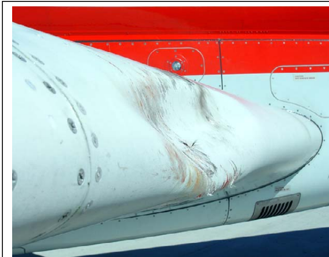
An Embraer ERJ-135ER struck a double-crested cormorant (DCCO) at 13:35 (local time) at about 400 AGL and 170 knots while climbing and banking left after departure from an east coast USA airport on 31 March 2003. The aircraft returned to the airport for a precautionary landing with a large dent in the leading edge of the right wing. The DCCO population in North America increased at a mean annual rate of 10.5%, 1966–2002 (Dolbeer and Eschenfelder 2003).
